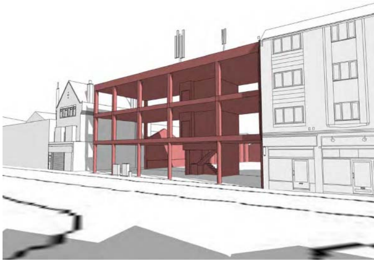
Retained Structure Shown in Red
